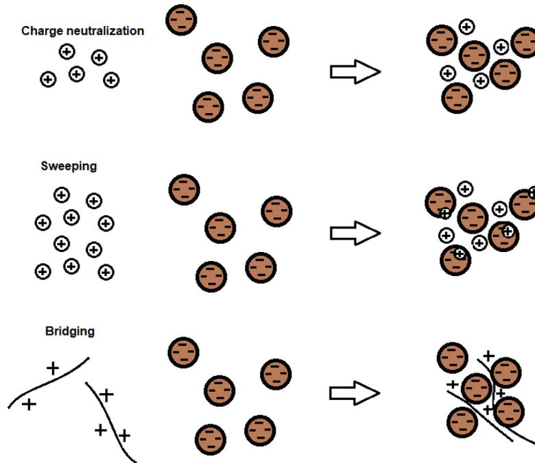
Figure 4: Mechanisms during charge neutralization, sweeping and bridging
