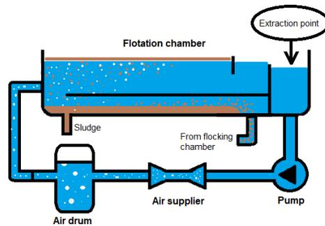
Figure 14: Extraction point of PFAS samples for the DAF outgoing water
