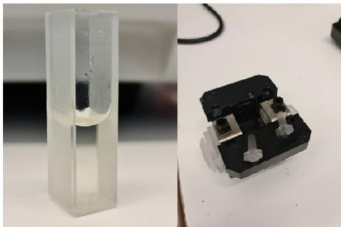
Figure 12: Size cell and Flow cell
