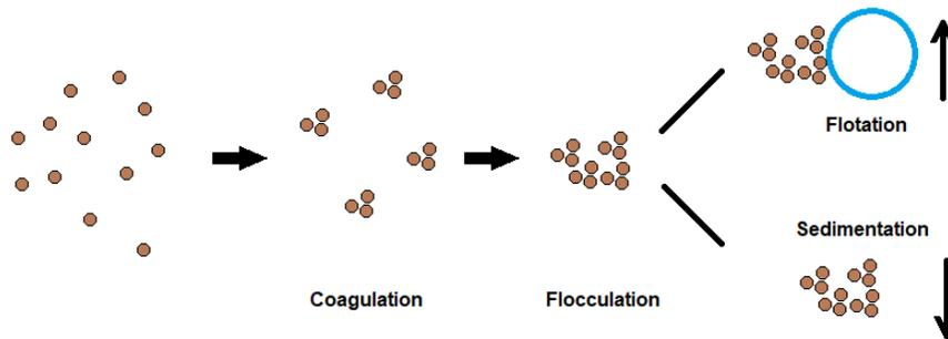
Figure 3: Coagulation and flocculation mechanisms
