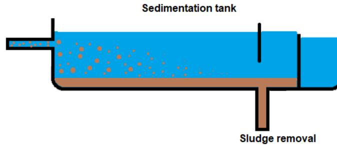
Figure 7: Simplified illustration of a sedimentation tank
