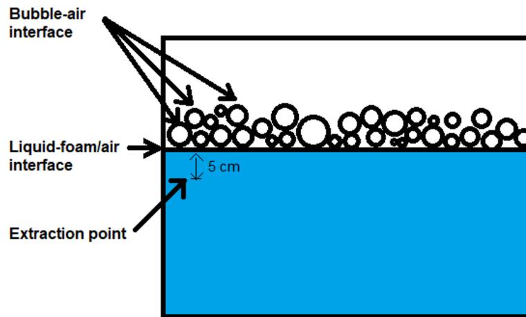
Figure 16: Extraction point for sample "Under surface, flotation foam"
