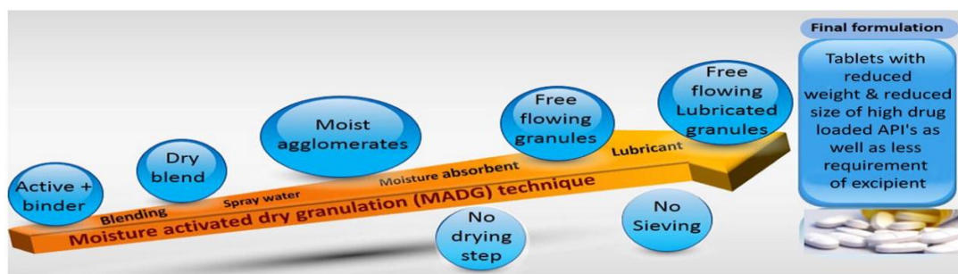
Figur 8. Fuktaktiverad torrgranuleringsmetod (MADG) process (Moravkar et al.,2017).
